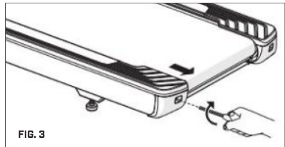
TIGHTENS LEFT SIDE OF ROLLER
